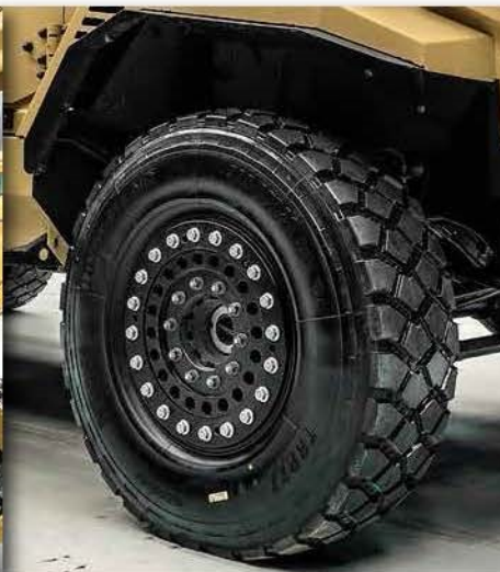
Upgraded Tires & Rims with Runflat Inserts
