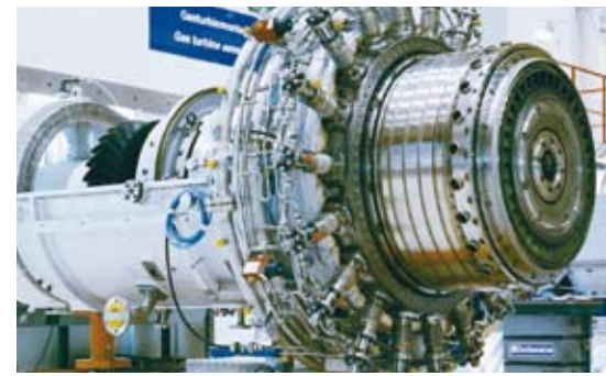
SGT-600 gas generator.
