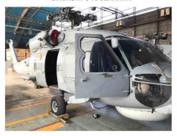
We are offering Seahawks featuring an S-70 airframe with Navy - specified avionics and a rescue hoist on the starboard side.
