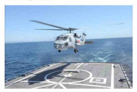
The S-70 Seahawk is specifically designed for ship borne operations. They feature a strengthened gear configured for smaller spaces, a folding tail and quick fold blades.
