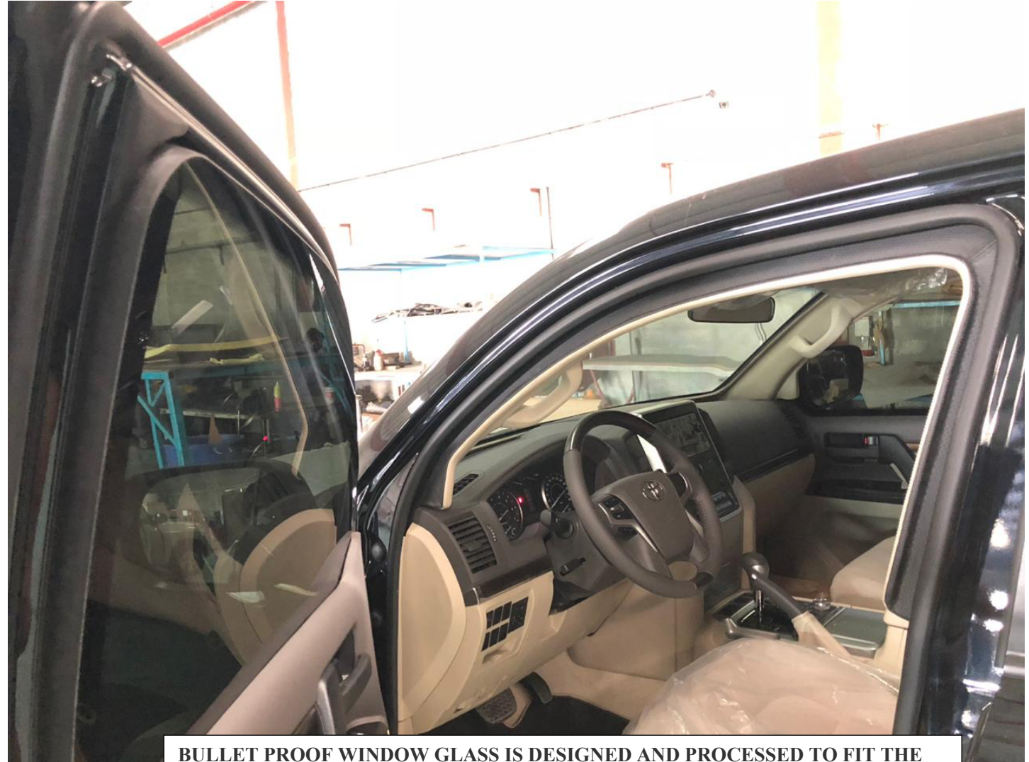
BULLET PROOF WINDOW GLASS IS DESIGNED AND PROCESSED TO FIT THE OVERLAPPING MOUNTED TO PILLARS
