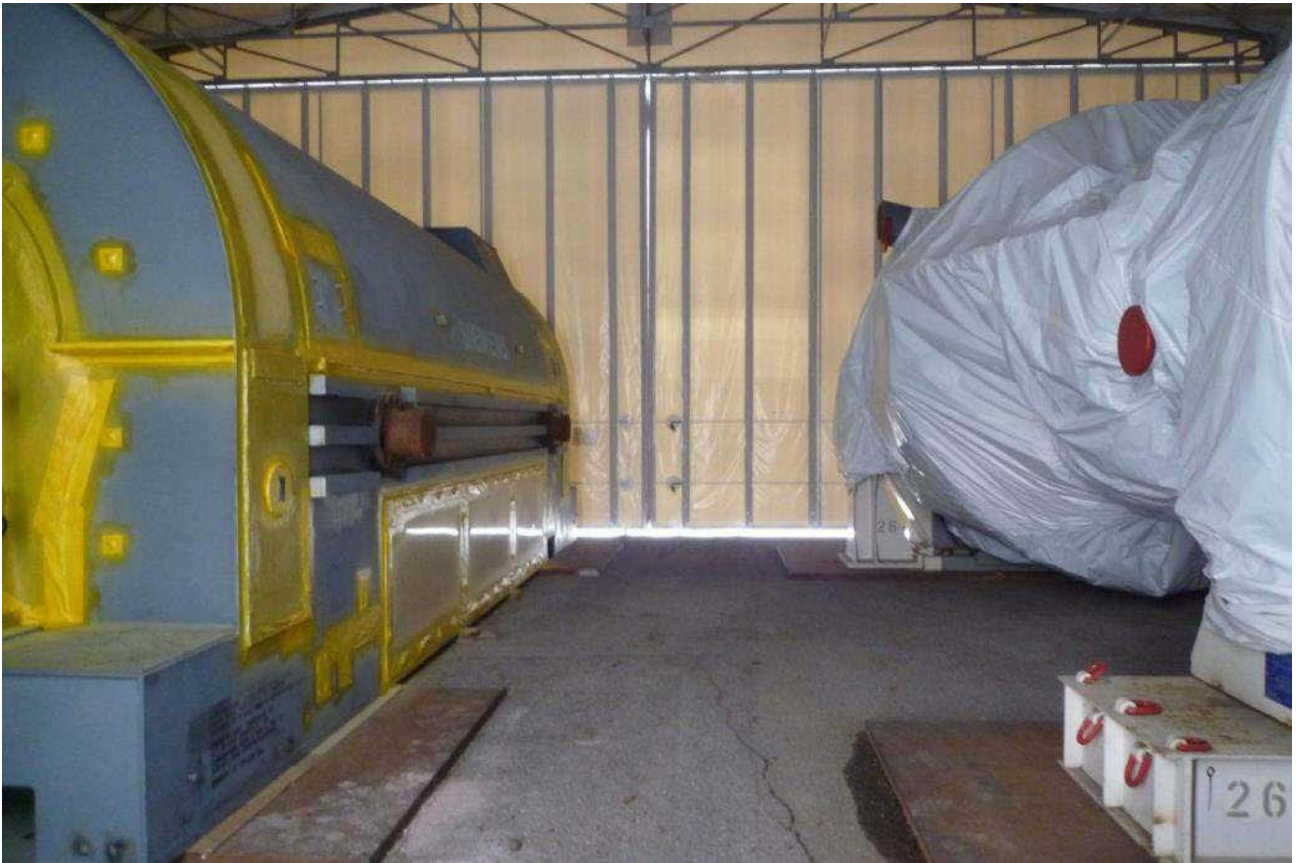
Figure 2: SIEMENS Gas Turbine SGT5-4000F &Generator SGen5-1000A
