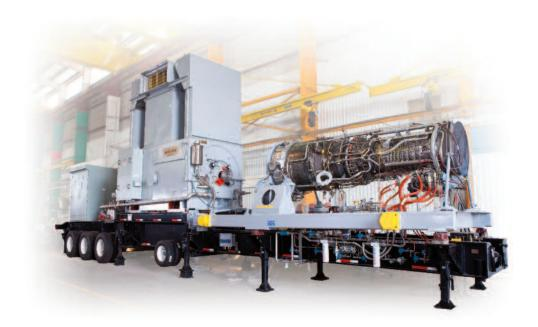
GE Power & Water now offers a faster, more reliable solution for bridging the gap between energy outages and dependable power generation. As the newest enhancement of GE's trailer-mounted unit, the TM2500+ offers a 31% increase in power in a more compact footprint with less time than ever between contract and commissioning.
