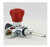
Y shape design, with safe self lock device to prevent inadvertent close due to hard knock or incorrect operation. Unscrew the switch hand-wheel by rotating in the counterclockwise direction, it is regarded as the open condition and close vice versa. There is safety diaphragm set in cylinder valve, with explosion pressure at (37-45)MPa to prevent the deformation and explosion of cylinder due to inner high pressure.
