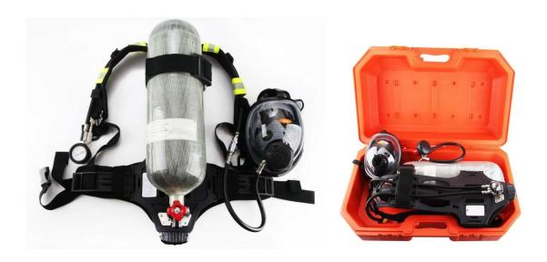
The self-contained positive pressure air breathing apparatus, which is a kind of isolated protective breathing equipment, provides respiratory protection for users working in oxygen-deficient environment or the environment with toxic and harmful gas. Under normal conditions, the pressure in the respirator mask is a little higher than the pressure in external environment, which can effectively prevent external toxic and harmful gas from intruding into the mask, and guarantee the safety of users.
