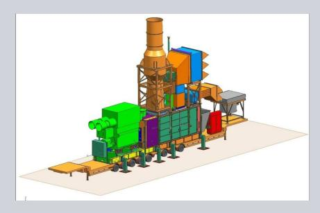
ISO performance will be as per SGT-400 data on SIEPEP based on the 12.9 MW ISO rating, however contract specific application needs to be reviewed by Siemens.
