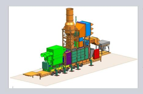
Trailer mounted SGT400 GTG package consisting of one trailer (3-axle) for GT driver package (standard SGT400) and one trailer (5 axle) for Generator and gearbox.
