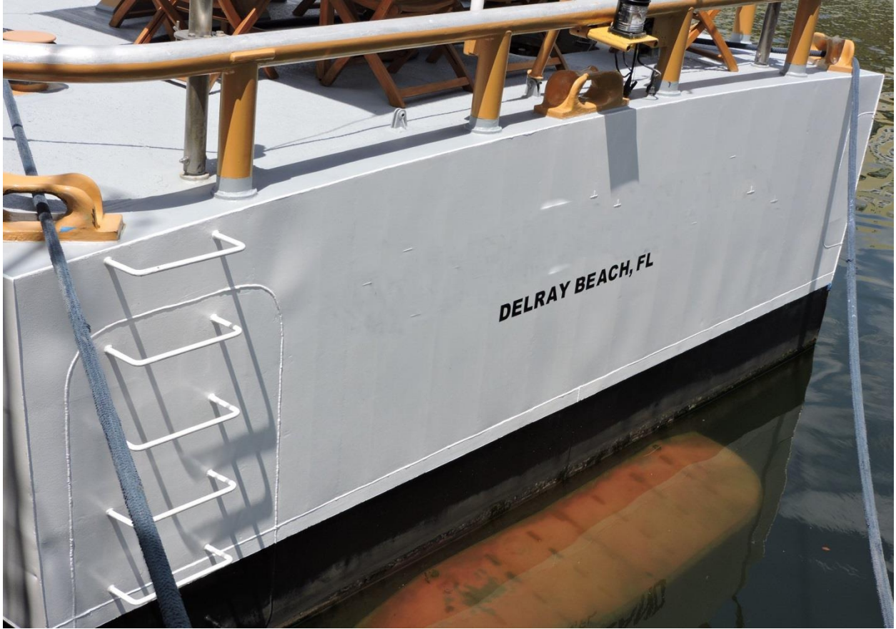
Stern appendage gives the ship a flatter ride and a 30% fuel savings. Additional cost .5 Million
