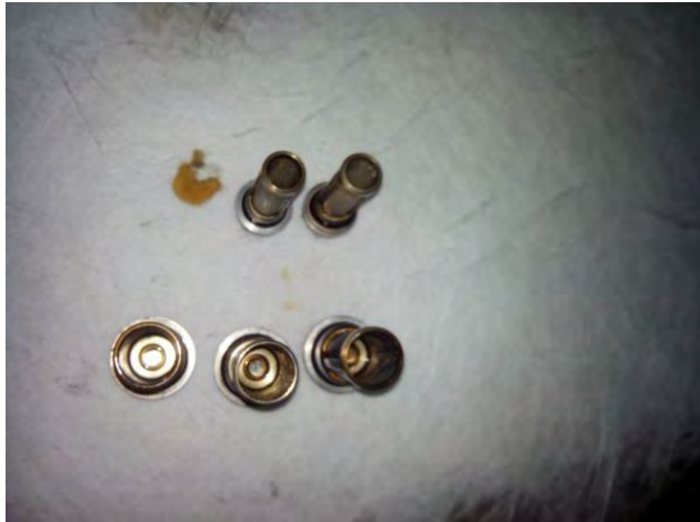
Picture 46: screen All screens and chip detectors clean. No remarks
