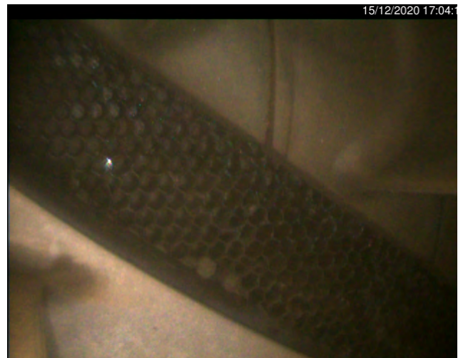
Picture 40: LPT stage 1 blades, sealing
