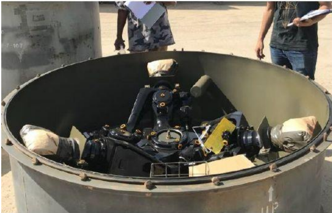
New Rotor Hub Stored in Special Steel Container
